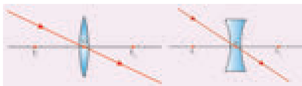
Figure 2.3 Rays passing through the optical centre
