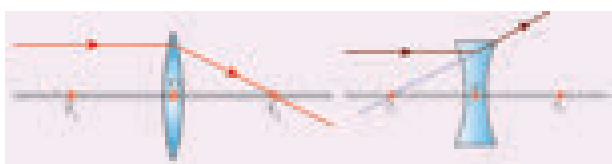
Figure 2.4 Rays passing parallel to the optic axis
